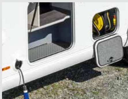
⊕ Self-retracting cable reel with 15 m of cable and central supply system
