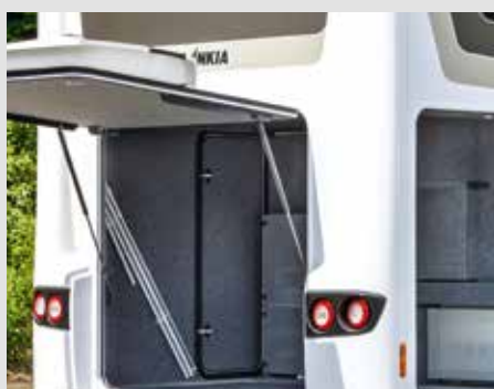
⊕ Adjustable rear and side flaps for loading and unloading the storage compartment
