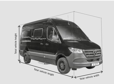
The **total vehicle length** corresponds to the measurement between the outermost point of the front spoiler and the outermost point of the rear panel (without trailer coupling).
